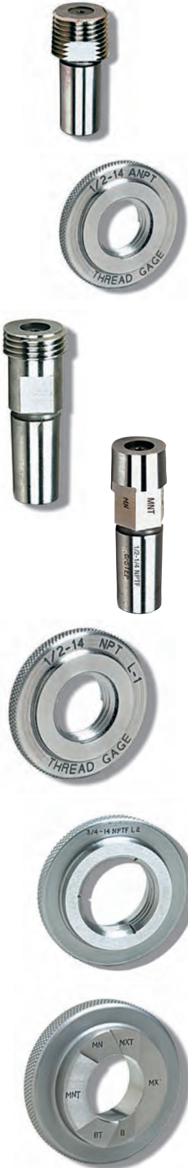
Fig. 1 Gaging internal American National Taper pipe threads with working gage. When the internal thread is chamfered, the gaging point shall be the intersection of the chamfer and the pitch cone of the thread.
